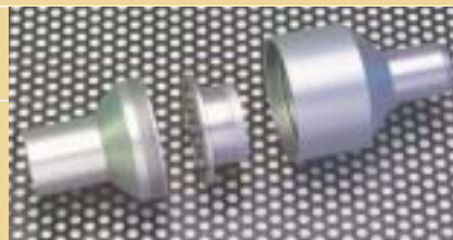
Exploded view - WINS impactor for PM 2.5 sampling
